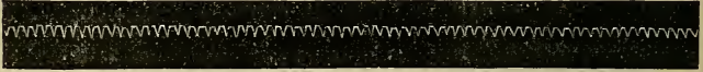
FIG. 8.—Signals obtained by the apparatus of Deprès, acted upon by an interrupting tuning fork of 500 vibrations per second. (Marey.)
